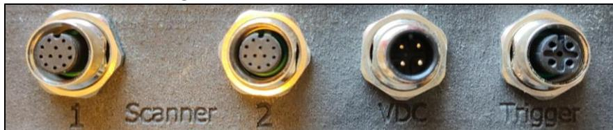
The scanner ports connect to 12 pin M12 male connectors (the two connectors on the left on the picture above), while the trigger (sensor) connector connects to a 5 pin M12 male connector, which can be seen on the right. If you got an externally powered Scannerbox, you will also notice the VDC connector between the sensor, and scanner connectors. This connector accepts a 4/5pin M12 female connector.
